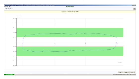
Three consecutive cycles will be performed, each with a higher flow rate than the last. Once the final highest flow rate cycle has been performed, click 'Done' and the calibration check results dialog will be shown.
