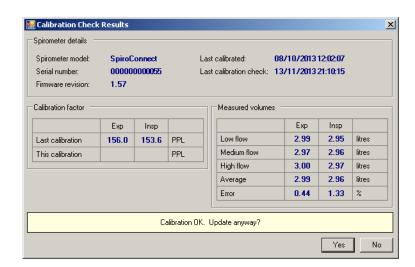
The procedure just performed is considered a calibration check if the results are reported as 'Calibration OK', and 'No' (in response to 'Update Anyway?') is clicked.
